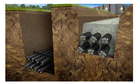
Thermaflow™ enables optimization of duct bank design for cost savings.
