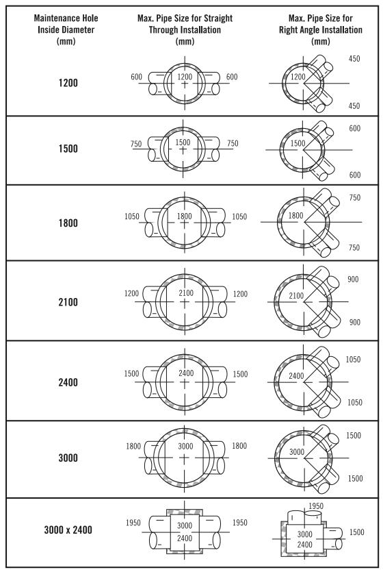
Note: Sizing shown is only for concrete pipes. All other pipe connections would need confirmation by Lafarge.
