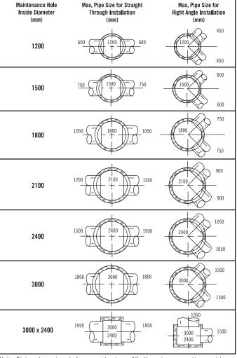
Note: Sizing shown is only for concrete pipes. All other pipe connections wuld need confirmation by Lafarge.
