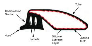
Self-Lubricated Gaskets are included with pipe material. If extra gaskets are required, an extra charge will apply.
