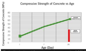
Typically designed for compressive strength of 35MPa, however it normally achieves 50-70 MPa at 28 days
