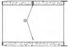
Lafarge can produce concrete pipe in a variety of sizes for trenchless installation with the jacking or tunneling methods. The pipe sections are designed for the additional axial force encountered in these operations and can be produced with ports for grout or lubrication.
