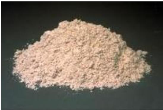
**Figure 1 Slag Cement (ground granulated blast furnace slag)**
