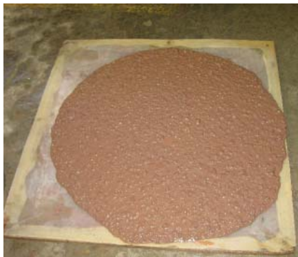
A flow test performed on UltraSeries™ Heavyweight prior to the pour demonstrates the self-consolidating nature of the concrete mix.
