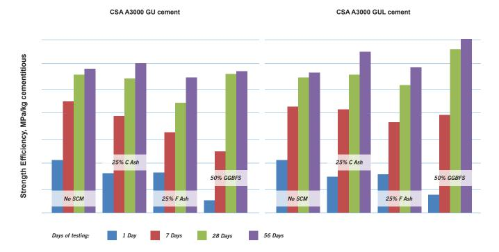
Data adapted from "Shrinkage and Durability Study of Bridge Deck Concrete," MS DOT State Study 216, Burns Cooley Dennis, Inc.; Dec. 2010; concrete strength comparison of RS mixes, agg source #1. The performance of individual material combinations may vary. Testing is recommended to determine their performance characteristics.
