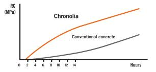
\*Chronolia is flowable up to 120 minutes after batching, depending on application. It is not a self consolidating concrete (SCC). \*\*Strength gains may depend on local conditions and materials available. Concrete curing conditions must be compliant to CSA A23.1.14.
